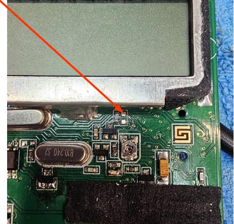
5. Connect a short ( 62mm) piece wire to potentiometer left pin.
