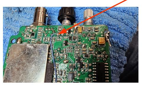
6. Connect the other side of the wire to the 3rd pin from the left, bottom row of the female header.
