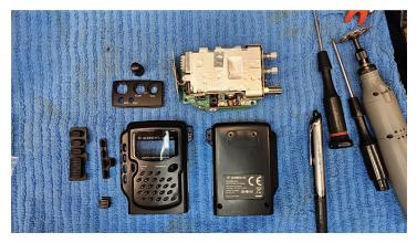
2. Remove the aluminum heat sink plate.
